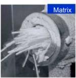
The liquid CO2 evaporate making CO2 snow, this is compressed by a piston then extruded as pellets.
